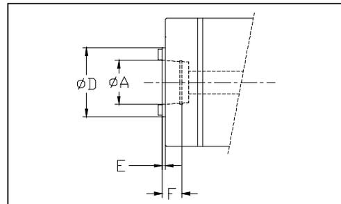
\* Minimum front bearing bore size [mm]
