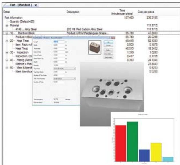
**The Costimator software from MTI Systems Inc. offers a knowledge base and the ability to do feature, product, and parametric-based costs analysis.**
